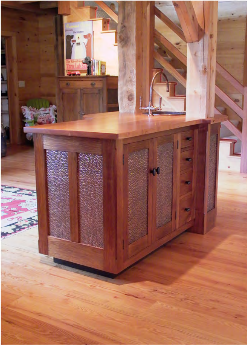
WET BAR ISLAND Scrub-plained butternut (mahogany stain), cherry top, copper panels and sink, bronze faucet & pulls
