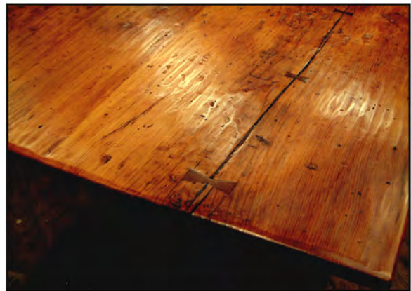
DETAIL OF TOP Salvaged pine Scrub planed surface Inlaid walnut butterfly keys
