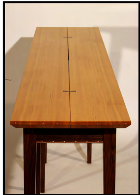
END DETAIL Two-plank top with gap Walnut butterfly keys
